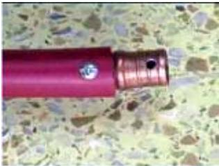
1. Dura PEX tubing usually comes in 25 ft spools. Cut the tubing into two 12.5 ft pieces; this will be enough for two 4-foot diameter frames. Insert the 1/2" male/male joint into one end of the tubing and drill a hole through both pieces with a power drill about 0.5" from the end of the tube. Insert the other end of the joint into the opposite end of the tube and repeat.
