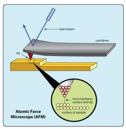
The probe of the AFM is a flexible cantilever—think of a diminutive diving board—with a tip attached to its underside. As the tip scans the sample, the force between them is monitored. To keep the force constant, the cantilever is moved up and down. A detection device, usually a reflected laser beam, measures the vertical movement of the cantilever, which corresponds to the hills and valleys of the sample's surface. A computer translates this vertical movement into an image.
