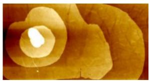
**IBM in xenon atoms:** This striking image taken by Ming Lee Tang at Stanford University shows a very thin crystalline film composed of stacked "terraces" (a 45-nanometer-thick layer of an organic semiconducting compound, a fluorenethiophene-oligomer).
