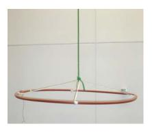
1. Hang the frame with the climbing rope and adjust inner ropes to make the frame level.
