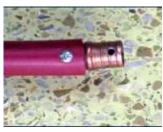
1. Dura PEX tubing usually comes in 25 ft spools. Cut the tubing into two 12.5 ft pieces; this will be enough for two 4-foot diameter frames. Insert the 1/2" male/male joint into one end of the tubing and drill a hole through both pieces with a power drill about 0.5" from the end of the tube. Insert the other end of the joint into the opposite end of the tube and repeat.
