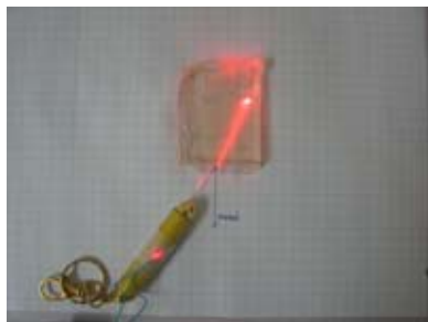
Beam of light is refracted as it enters the gelatin.
