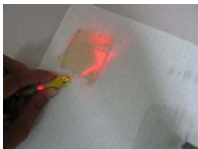
Loss of light due to grooves on the sides of the gelatin.
