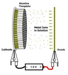
the following procedure you will use a liquid metal (Gallium Indium Eutectic) for contact and a AA battery to force the plating of nickel into the pores.
