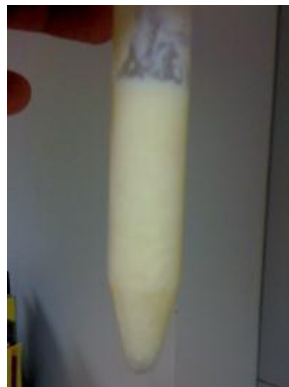
Control test—egg not soaked in polluted water. There is no color, so there is no presence of mercury.
