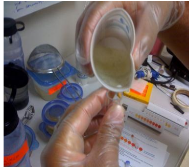
Use the HMT mercury test to test the polluted water
