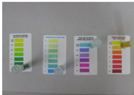
Step 4: Test the distilled water sample using a test kit for the initial, unpolluted conditions.
