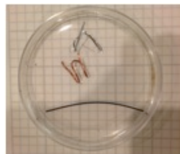
Wires in contact with hot water.
