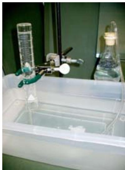
Collecting gas by water displacement
