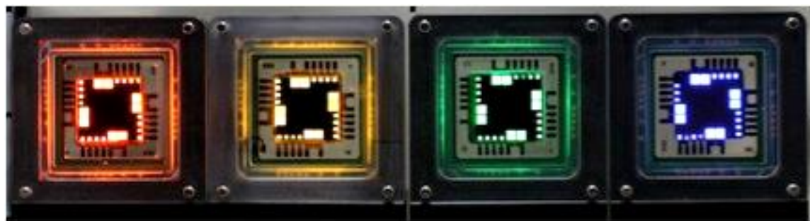
Figure 3: Quantum Dot based Light Emitting Diodes (QLEDs) are currently being developed for displays and lighting applications. In the photo above, we are seeing QLEDs manufactured by QDVision. Image at: http://www.qdvision.com/qleds-the-future .
