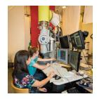
**Transmission Electron Microscope (TEM):** TEMs shoot electrons through thin samples and look at the electrons that have reached the other side. Even though TEMs are large and expensive, they are actually similar to overhead projectors, since both produce 2D "shadows" of a sample. TEMs have incredible resolution, so it's possible to image individual atoms with a TEM! TEMs were invented in 1931 by Ernst Ruska and Max Knoll. TEMs cost between \$400K and \$4M!
