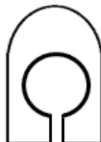
Well and Channel (depth = 3-4 mm) for IPA boat only
