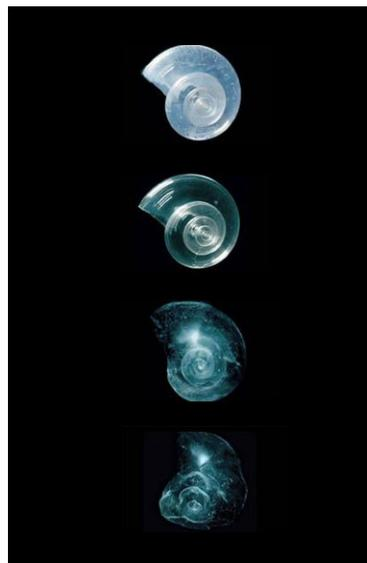
**A sea snail shell dissolved in acidic salt water over the course of 45 days during a lab experiment**
