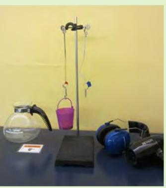
Holder with different color coded labels for nitinol and steel springs. Memory wire for additional experimenting.
