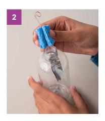
Experiment with the model *electroscope*— an instrument used to detect electrical charge. First, rub the foam tray on the wool felt for about ten seconds to charge it up. Then, wave the tray next to the wire on top of the electroscope without touching the tray to the wire. What do you notice about the foil shapes inside?
