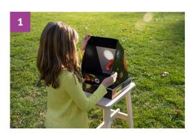
Point the Solarscope at the Sun, and move or tilt the box until the small mirror reflects the Sun's image onto the white screen at the back of the box.
