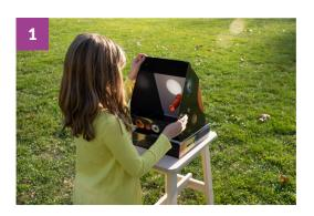
Point the Solarscope at the Sun, and move or tilt the box until the small mirror reflects the Sun's image onto the white screen at the back of the box.
