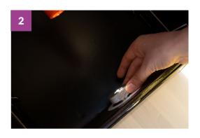
Focus the Solarscope by slowly rotating the mirror until the projected image of the Sun is clear and has crisp edges.
