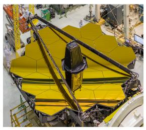
The Webb telescope's iconic gold mirror array is actually made of 18 interlocking, foldable segments.
