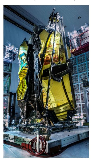
The James Webb Space Telescope's massive mirror folds up for launch and then unfolds once in orbit.
