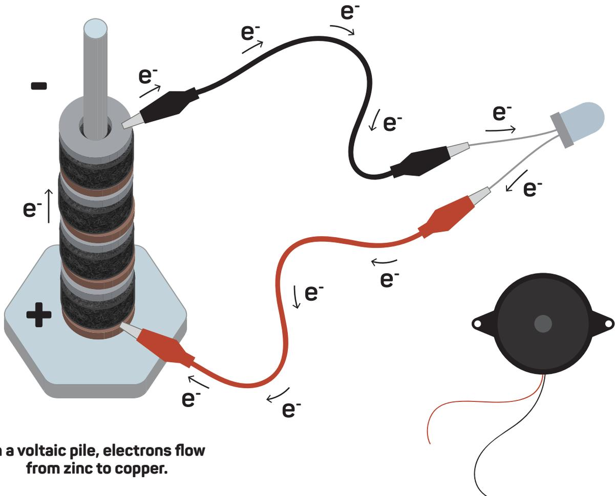
In a voltaic pile, electrons flow from zinc to copper.
