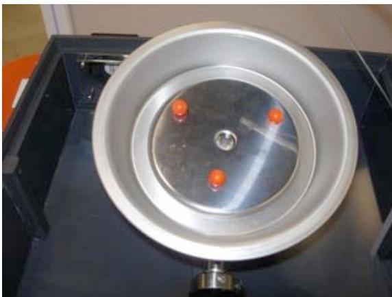
Secure the leaf to the steel plate with the three magnets.
