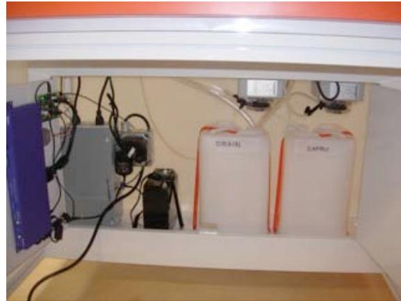
Orient the jug as shown, and return the two water supply lines with their weighted strainers back into the tank. Screw the cap down.
