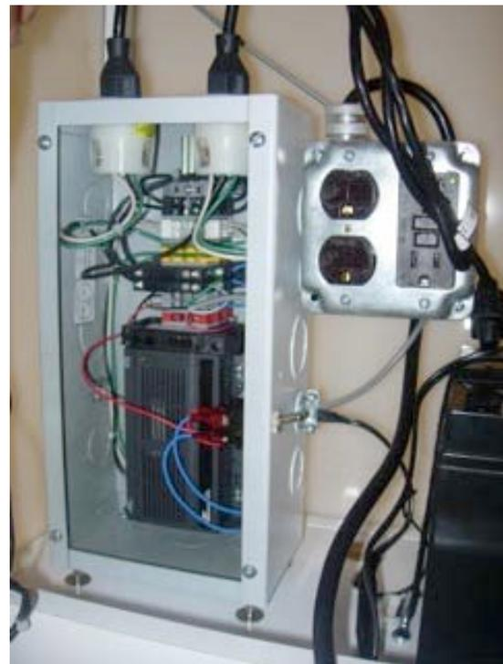
The output voltage is adjusted to ~13.3 VDC to charge the 18 Ah sealed lead acid battery (McMaster Carr #7448K76)
