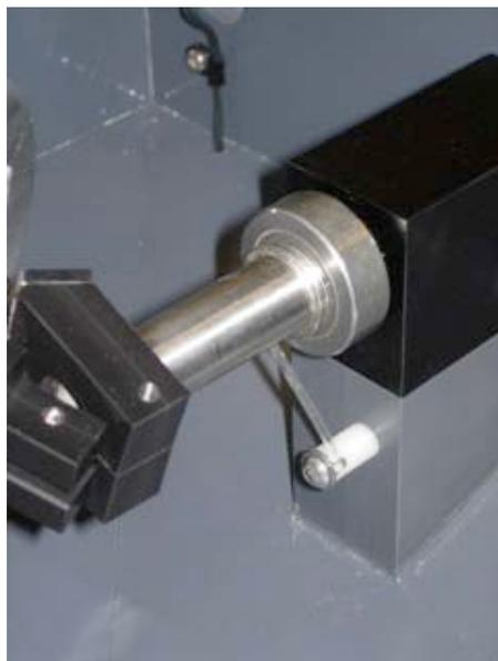
The pans are tipped to the side by a short length of urethane round belting acting as a spring. The tension can be adjusted by loosening the aluminum shaft collar and turning it to either increase or decrease the tension on the belting. Once the desired tension is achieved, tighten the shaft collar again.
