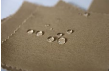
Water on nano fabric Gary Hodges for the NISE Network CC BY-NC-SA 3.0
