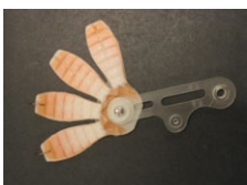
Gecko robot foot Mark Cutkosky, Stanford University
