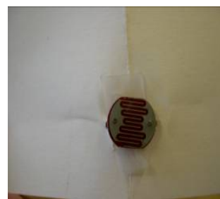
Above: photodetector taped to a folded index card
