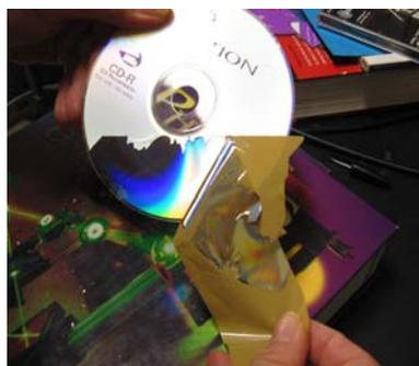
Peel off the label and reflecting layer
