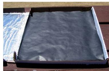
6. Fold your pizza box into a box shape by folding along the creases of the box. Because we do not want heat loss by *convection*, we will use duct tape to tape the edges of the pizza box shut so that air can not escape the box.
