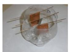
**Figure 3: Electrodeposition** Chamber
