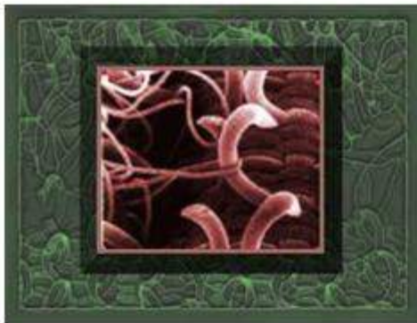
Scanning Electron Microscope (SEM) Image of Velcro Courtesy www.about.com
