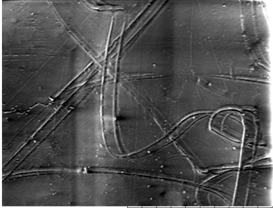
TM3000_0154 2012/07/19 11:21 F D7.9 x1.8k 50 um Scratched CD 1800x
