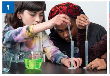
Use the pipette to add 4 mL of highlighter water to two graduated cylinders.
