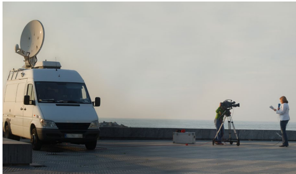
A satellite TV truck parked on a city street sends radio waves to space to be distributed across the globe.
