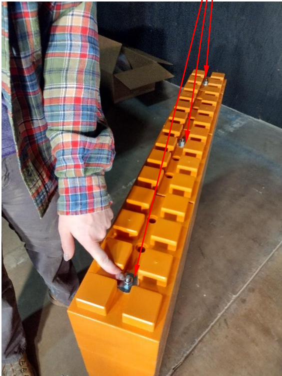
3/8" Hex Nut and Fender Washers at Short Leg Assembly (3 each)
