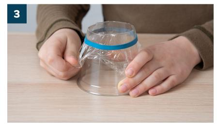
Fasten the plastic wrap so that it is evenly taut, like you might imagine on a drum. Now wrap the rubber band around the tube to secure the plastic wrap in place.
