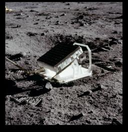
Apollo 11 astronauts placed this array of mirrors on the Moon. By bouncing lasers off these mirrors, scientists on Earth can very accurately measure the distance to the Moon.
