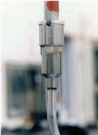
An electrostatic discharge point on the Sojourner Mars rover's antenna.
